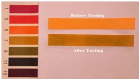
Fig. 6 Manual Testing of soil Fertility (pH) using Universal Indicator paper
